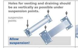
Missing holes for venting and draining on hollow sections can cause dangerous explosions!
